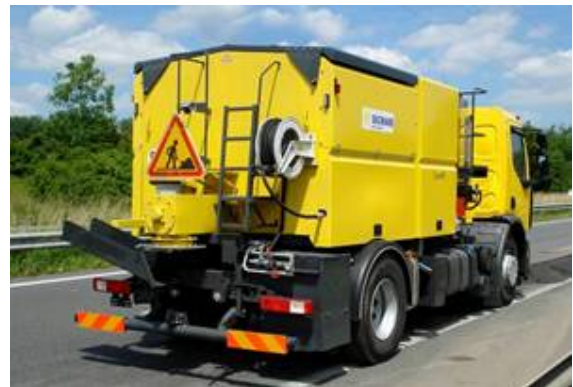
SWIFT (pothole repairs)
