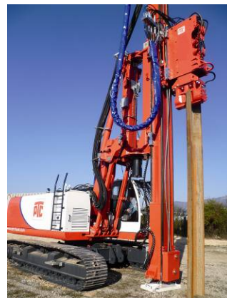
PR20 piling rig
